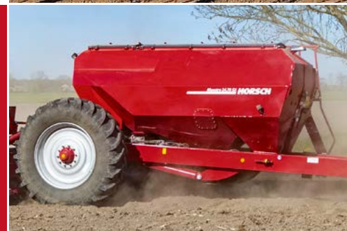
Seed wagon with a capacity of 2 000 litres for seed and 7 000 litres for fertiliser for Maestro 24 SV/SX und 36 SV
