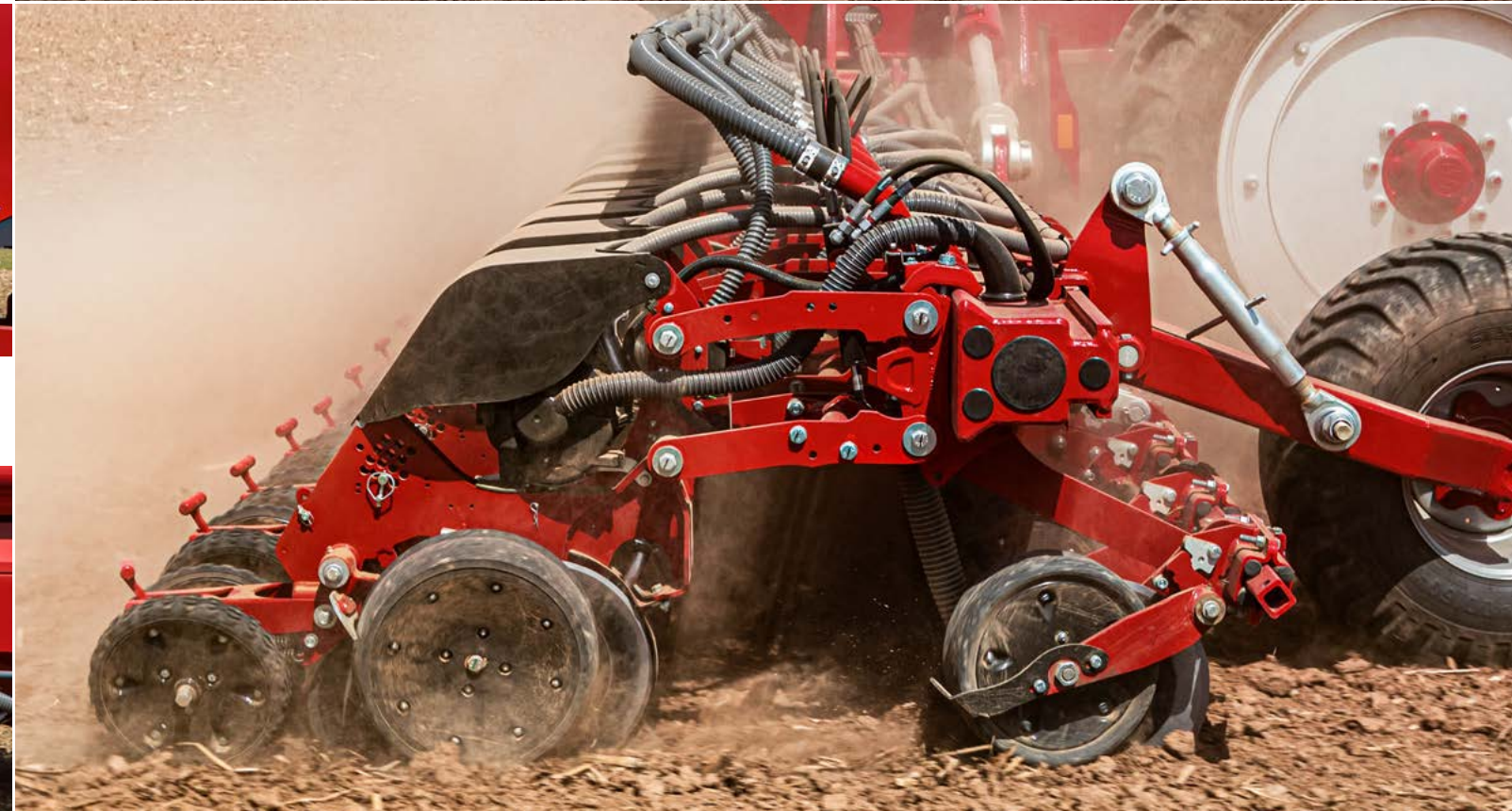
SingleDisc fertiliser coulter suspended at the coulter shaft as well as heavy and solidly built row of the Maestro SV/SX with precise grain singulation and Main Tank Supply System (MTS)
