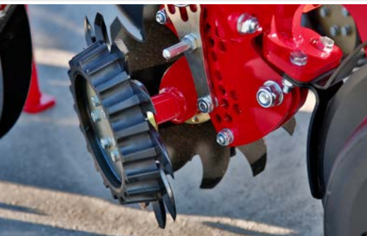
Optional trash wheels, floating with depth control
