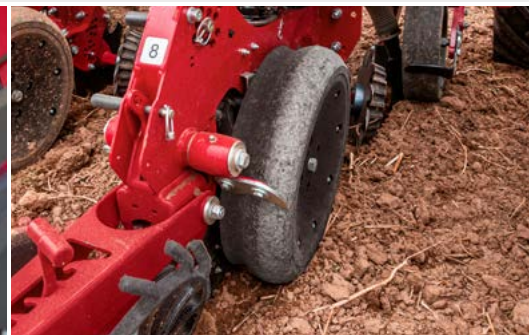
RID wheel reduces soil compaction directly at the seed slot in very hard or no-till conditions
