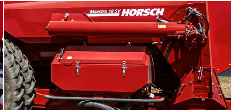
Filling auger and central micro-granular unit with a capacity of 400 resp. 500 litres
