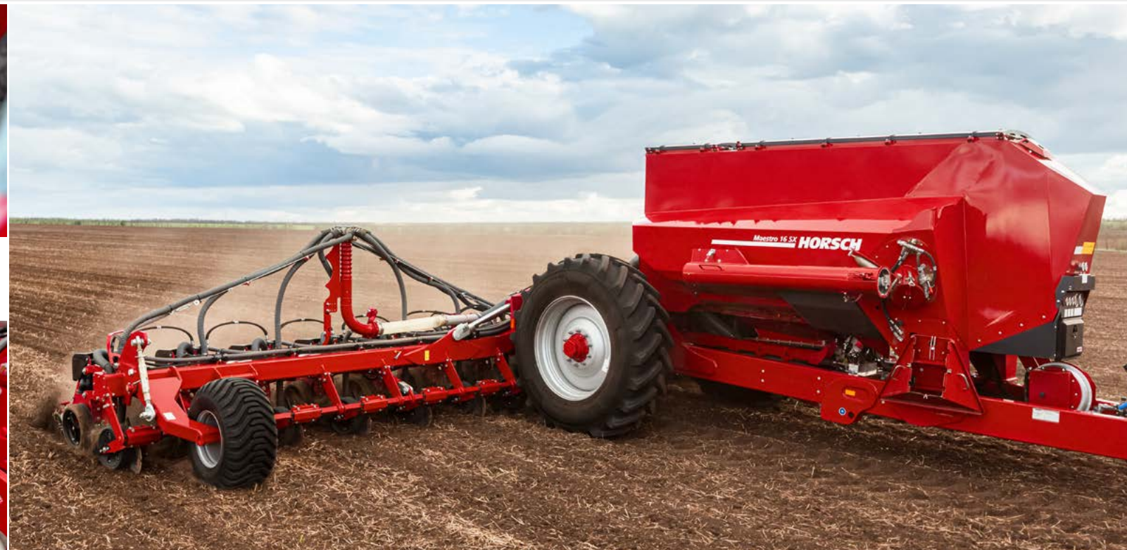
Maestro 16 SX with 5 400 litres of fertiliser and 2 200 litres of seed
