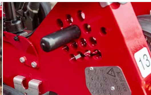
Hole pattern for depth adjustment with 14 steps
