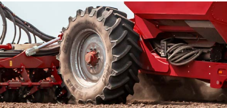
Tyres 580/70 R 38 with large diameter and large contact area
