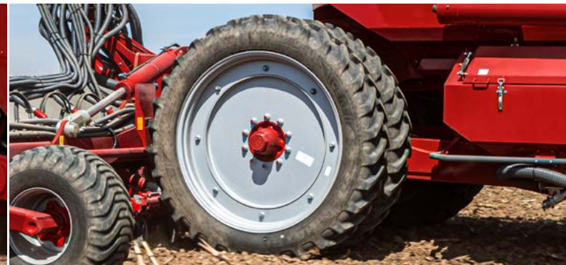
Twin tyres 300/95 R 46 for 45 cm and 50 cm row spacing
