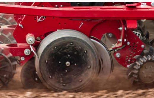
Heavy DoubleDisc couler with low-wear, stable depth control
