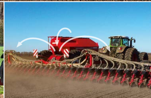
Transfer of the seed wagon weight to the seed bar for a higher coulter pressure and a release of the wheels
